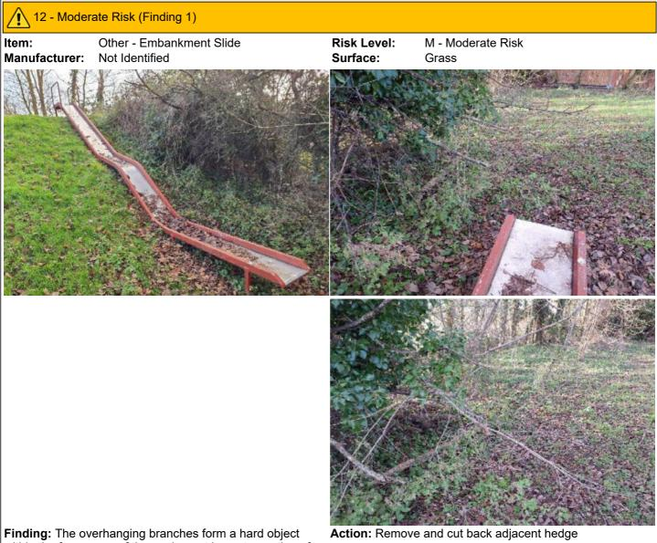
**Finding:** The overhanging branches form a hard object within the free space of the equipment in contravention of the requirements of BS EN 1176 Part 1
